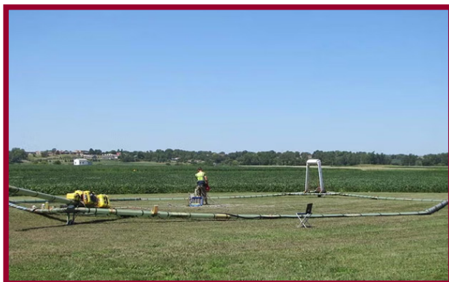
Preparing the hoop-shaped geophysical device for surveying. Photo from Lewis and Clark Natural Resources District, Nebraska.
